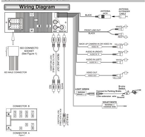
ISO CONNECTOR 4PIN+8PIN FEMALE WITH MALE TERMINAL
