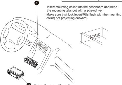
Secure the rear of the unit. After fixing mounting bolt and power connector, fix the rear of the unit to the car body by bubber cushion.
