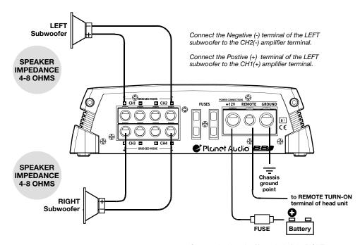
Connect the Negative (-) terminal of the RIGHT subwoofer to the CH4(-) amplifier terminal.
